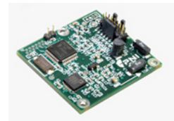
Figure 4.4 PNI digital compass
